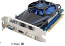
Crysis 3, for example, the 7750 and 7730 scored 27.4 and 21.2fps respectively. In Bioshock, the figures were 40.9 and 33.5fps, and in Stalker, 45.5fps played 37.3fps. These scores are playable, suggesting that the 7730 isn't a total write-off as a gaming card.
