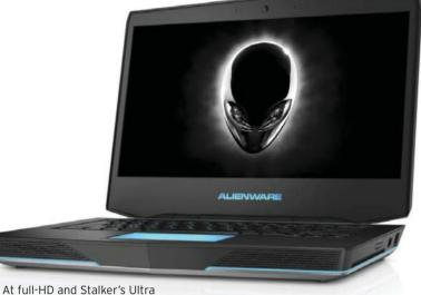
There's plenty to like about the IPS panel. The matt finish banishes reflections that hamper gaming, and it's matched with a high resolution – our model has been upgraded with a full-HD screen. Quality is high: the measured brightness level of 325cd/m² ensures punchy images, and a reasonable black level of 0.29cd/m² lends games and movies real depth. The contrast ratio and viewing angles are both good, although the matt layer adds more grain than we'd like.
